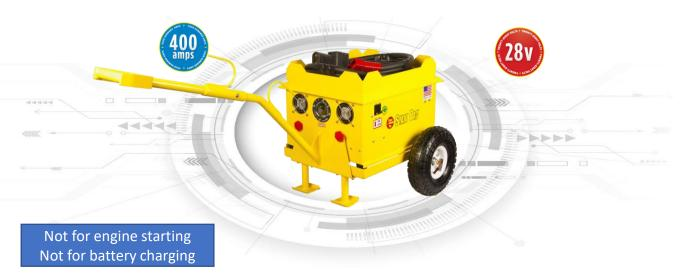
The START PAC® model 53400 - 24/28V is the most powerful power supply. It has been designed to power up 24 Volt aircraft systems and will continuously deliver up to full 400 amp DC output. The voltage output is set to 28 Volts to simulate the same voltage as when the aircraft is running under power.
