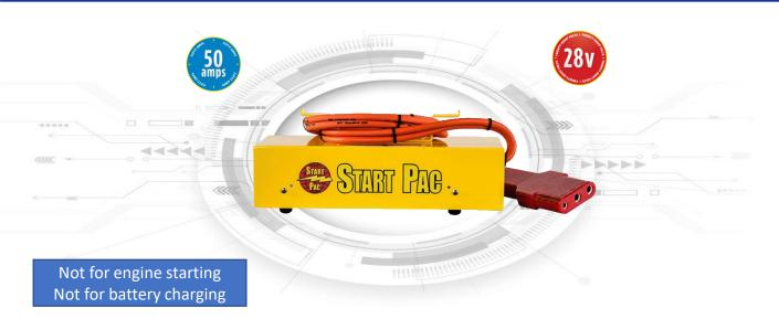
The most commonly used 24V portable power supply, this START PAC<sup>®</sup> model has been designed to power up 24 Volt aircraft systems and will continuously deliver up to full 50 amp DC output. The voltage output is set to 28.5 Volts to simulate the same voltage as when the aircraft is running under power.
