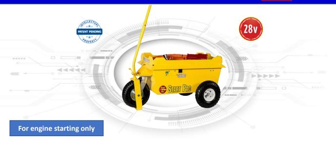
The START PAC® GPU model 3328 Special is designed to perform repeated superior starting functions for large turbine engines, including the Garrett TPE 331. It is rated at 2800 peak starting amps and is a full 28 Volt battery pack (28.5 Volts to be exact, 30.5 volts at rest).
