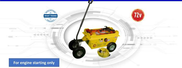
START PAC<sup>®</sup> carries the leading railroad locomotive starter unit on the market. This American made Patent Pending lightweight 72V mobile ground power unit is designed to directly start the locomotive engine when the locomotive battery is not sufficiently charged or capable of starting the engine. The 3324RR locomotive engine starting unit can be manufactured with wheels or without wheels to be truck mounted.
